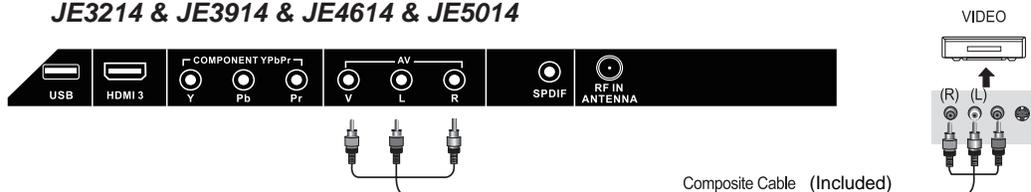
Connect the LED TV's Composite In terminal to VCR's Composite OUT terminal using the included Composite cable. (Make sure the color of the terminals and the colors of the cable are the same.)
