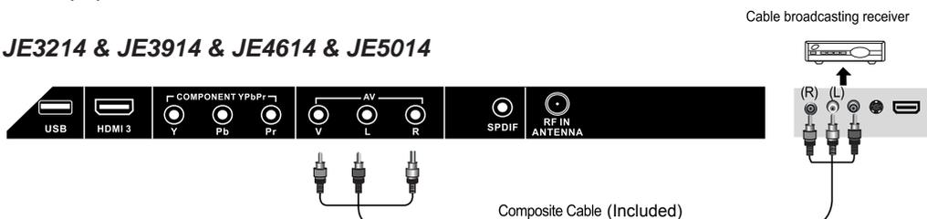
Connect the LED TV's Composite In terminal to the cable broadcasting receiver Composite Out terminal using the Composite cable. (Make sure the color of the terminals and the color of cables are the same)
